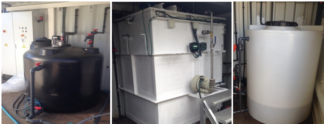
Figure 5 Pictures of feed storage tank (left), the MBR aeration tank (middle) and one of the permeate tanks (right)
